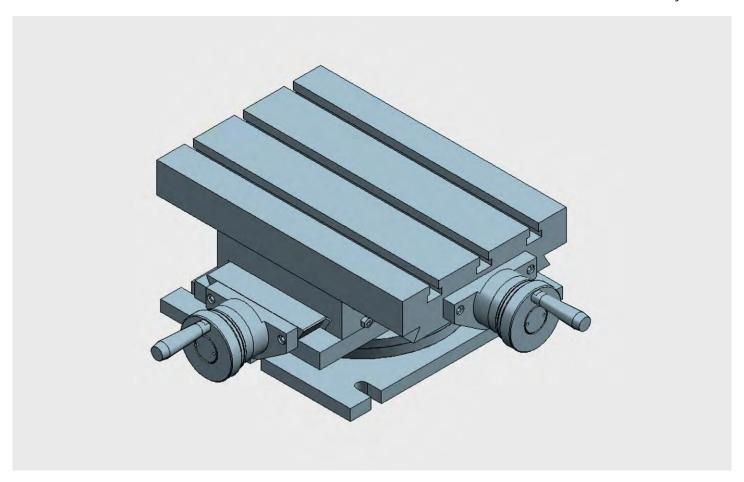
Double axis crosstable with rotary basis: the swivel support base comes with 180° in order to carry out angled works. All elements in stabilized cast iron GG25. All surfaces with grinded finishment. Millimetered rules in XY. Vernier/nonuis matt chrome. Dial, with zero setting. Spindle with trapezoidal thread. Adjustable spindle nut. Standard lock in XY (M6 screw to block the dovetailed guides in working position)
