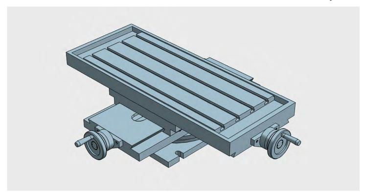
Double axis crosstable with rotary basis: the swivel support base comes with 180° in order to carry out angled works. All elements in stabilized cast iron GG25. All surfaces with grinded finishment. Millimetered rules in XY. Vernier/nonuis matt chrome. Dial, with zero setting. Spindle with trapezoidal thread. Adjustable spindle nut. Standard lock in XY (M6 screw to block the dovetailed guides in working position)
