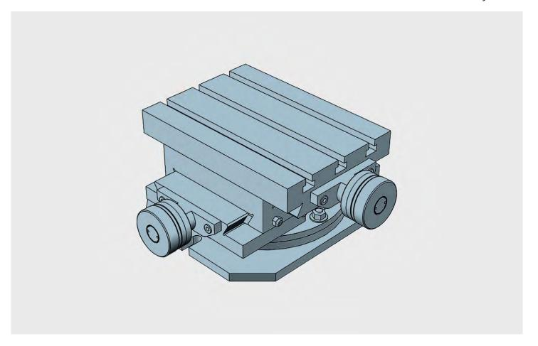
Double axis crosstable with rotary basis: the swivel support base comes with 180° in order to carry out angled works. All elements in stabilized cast iron GG25. All surfaces with grinded finishment. Millimetered rules in XY. Vernier/nonuis matt chrome. Dial, with zero setting. Spindle with triangular thread. Adjustable spindle nut. Standard lock in XY (M6 screw to block the dovetailed guides in working position)
