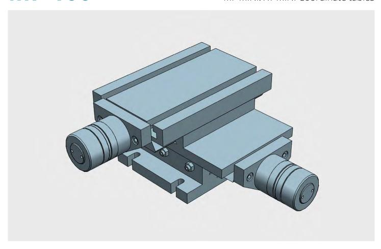
MINI fixed double axis crosstable: for applications in small mechanical operations, testing and metrology laboratories. Compact design and highly sensitive movements. All elements in stabilized cast iron GG25. All surfaces with grinded finishment. Millimetered rules in XY. Vernier/nonuis matt chrome. Dial, with zero setting. Spindle with triangular thread. Adjustable spindle nut. Standard lock in XY (M5 screw to block the dovetailed guides in working position)
