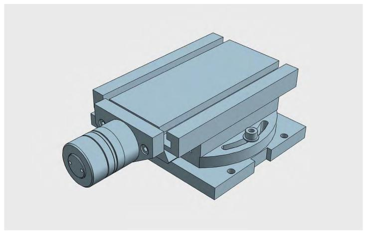
MINI single axis slide tables with rotary basis (60°) for applications in small mechanical operations, testing and metrology laboratories. Compact design and highly sensitive movements. All elements in stabilized cast iron GG25. All surfaces with grinded finishment. Millimetered rules in XY. Vernier/nonuis matt chrome. Dial, with zero setting. Spindle with triangular thread. Adjustable spindle nut. Standard lock in XY (M5 screw to block the dovetailed guides in working position)
