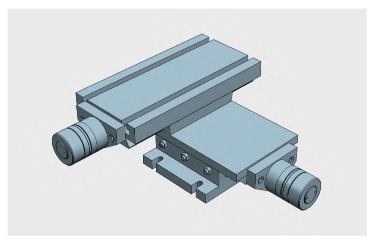
MINI fixed double axis crosstable: for applications in small mechanical operations, testing and metrology laboratories. Compact design and highly sensitive movements. All elements in stabilized cast iron GG25. All surfaces with grinded finishment. Millimetered rules in XY. Vernier/nonuis matt chrome. Dial, with zero setting. Spindle with triangular thread. Adjustable spindle nut. Standard lock in XY (M5 screw to block the dovetailed guides in working position)
