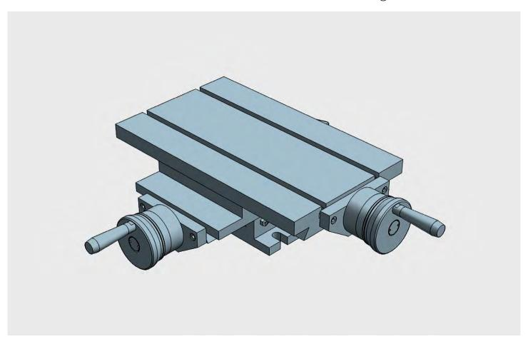
LIGHT Fixed double axis crosstable, designed to be used in light mechanical operations in which height of the table is a major factor All elements in stabilized cast iron GG25. All surfaces with grinded finishment. Millimetered rules in XY. Vernier/nonuis matt chrome. Dial, with zero setting. Spindle with triangular thread. Adjustable spindle nut. Standard lock in XY (Jaccard type)
