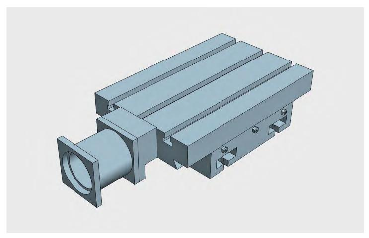
Single automatic X unit. All elements in stabilized cast iron GG25. All surfaces with grinded finishment. Ballbearing spindles with double nut. Dovetailed guides with turcite. Any CNC available under request
