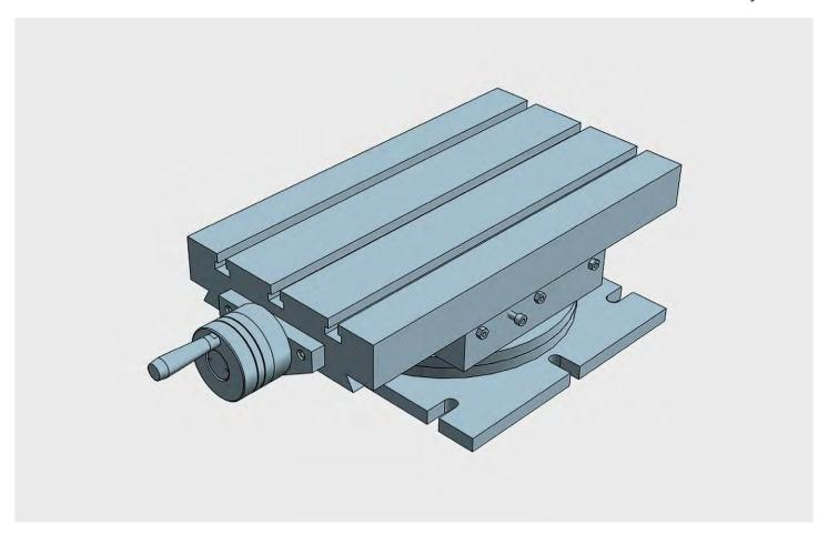
SINGLE axis table with rotary table (180°) for applications with linear units. Can be used in horizontal or vertical position All elements in stabilized cast iron GG25. All surfaces with grinded finishment. Millimetered rules in XY. Vernier/nonuis matt chrome. Dial, with zero setting. Spindle with trapezoidal thread. Adjustable spindle nut. Standard lock in XY (M6 screw to block the dovetailed guides in working position)
