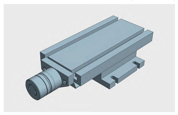
MINI single axis slide tables for applications in small mechanical operations, testing and metrology laboratories. Compact design and highly sensitive movements. All elements in stabilized cast iron GG25. All surfaces with grinded finishment. Millimetered rules in XY. Vernier/nonuis matt chrome. Dial, with zero setting. Spindle with triangular thread. Adjustable spindle nut. Standard lock in XY (M5 screw to block the dovetailed guides in working position)
