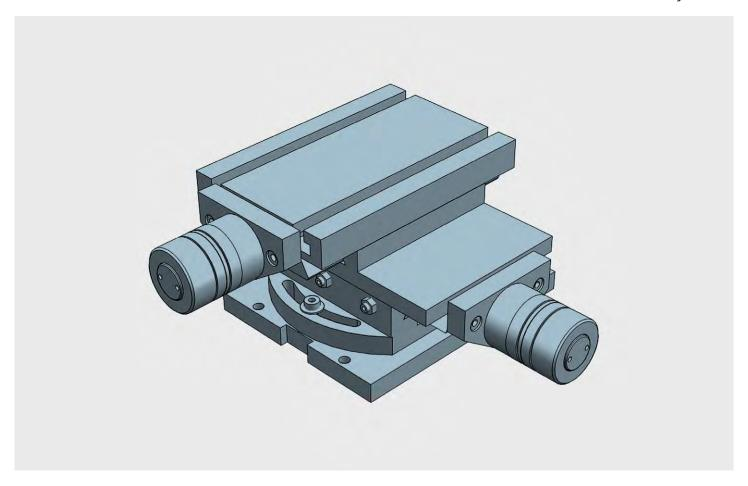
MINI double axis crosstable with rotary basis (60°): for applications in small mechanical operations, testing and metrology laboratories. Compact design and highly sensitive movements. All elements in stabilized cast iron GG25. All surfaces with grinded finishment. Millimetered rules in XY. Vernier/nonuis matt chrome. Dial, with zero setting. Spindle with triangular thread. Adjustable spindle nut. Standard lock in XY (M5 screw to block the dovetailed guides in working position)
