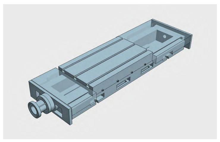
SINGLE axis table for applications with linear units. Can be used in horizontal or vertical positionAny CNC available under request All elements in stabilized cast iron GG25. All surfaces with grinded finishment. Ballbearing spindles with double nut. Dovetailed guides with turcite. Any CNC available under request
