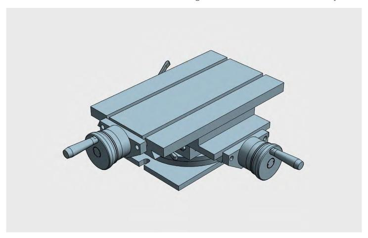
LIGHT double axis crosstable with turning basis, designed to be used in light mechanical operations in which height of the table is a major factor All elements in stabilized cast iron GG25. All surfaces with grinded finishment. Millimetered rules in XY. Vernier/nonuis matt chrome. Dial, with zero setting. Spindle with triangular thread. Adjustable spindle nut. Standard lock in XY (Jaccard type)
