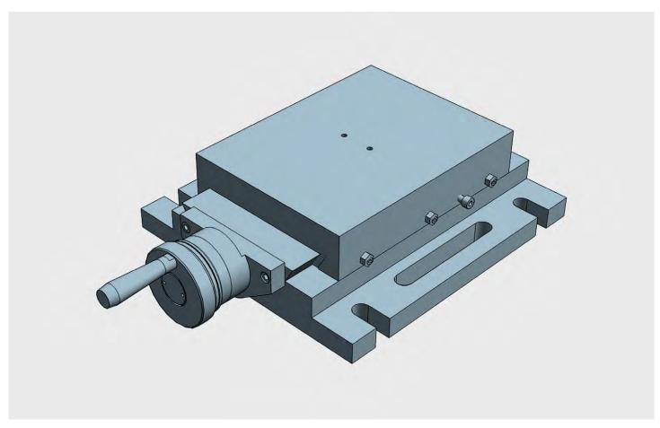
SINGLE axis table for applications with linear units. Can be used in horizontal or vertical position All elements in stabilized cast iron GG25. All surfaces with grinded finishment. Millimetered rules in XY. Vernier/nonuis matt chrome. Dial, with zero setting. Spindle with trapezoidal thread. Adjustable spindle nut. Standard lock in XY (M6 screw to block the dovetailed guides in working position)
