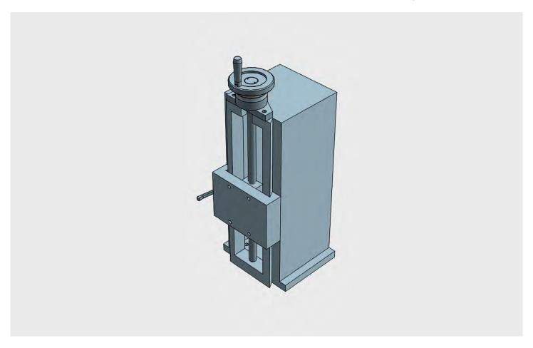
VERTICAL axis table for applications with linear units. Can be used only in vertical position All elements in stabilized cast iron GG25. All surfaces with grinded finishment. Millimetered rules in XY. Vernier/nonuis matt chrome. Dial, with zero setting. Spindle with trapezoidal thread. Adjustable spindle nut. Standard lock in XY (M6 screw to block the dovetailed guides in working position)
